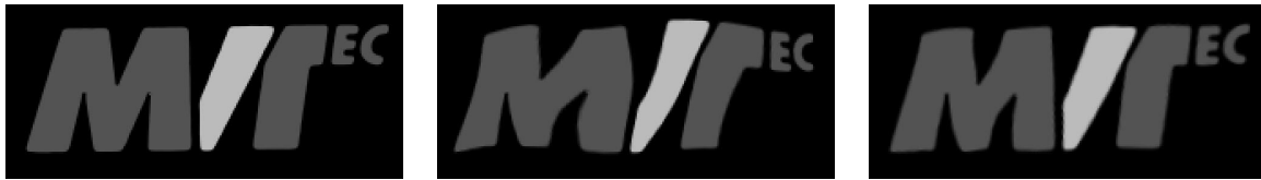
Figure 10.6: From left to right: template image, corresponding part of the search image, rectified image.
