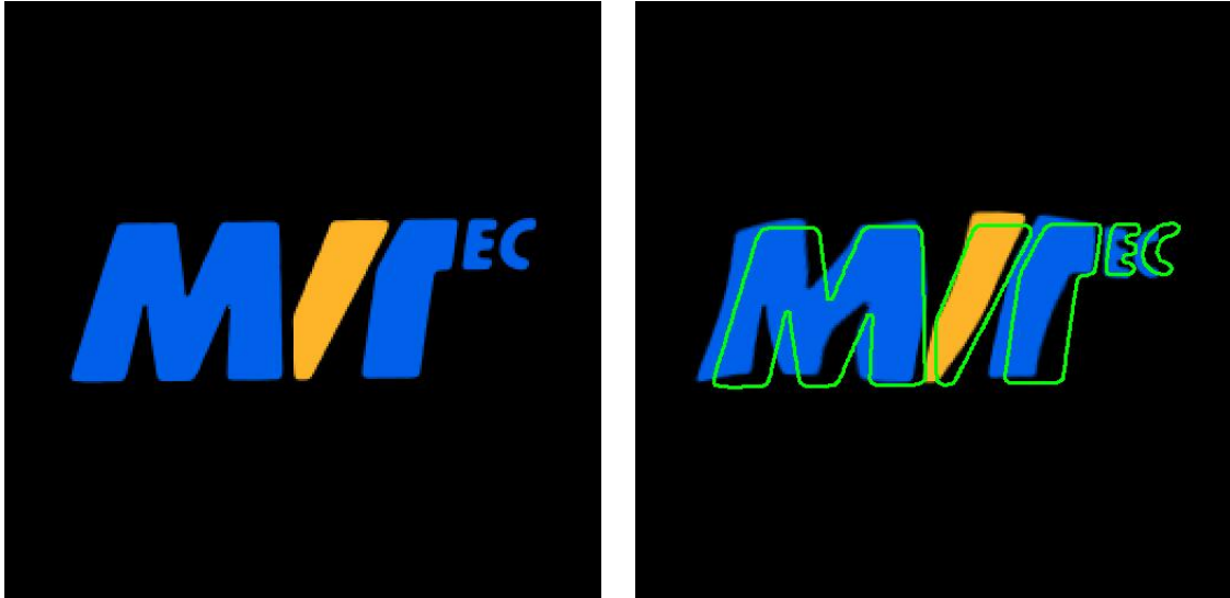
Figure 10.5: (left) “MVTec” logo used for the model creation; (right) deformed logo instance overlaid by the model contours.
