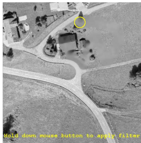
Figure 3.3: Partially filtered image.
