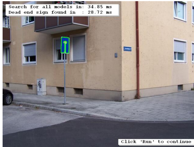
Figure 10.7: A dead end road sign is located via uncalibrated perspective deformable matching.
