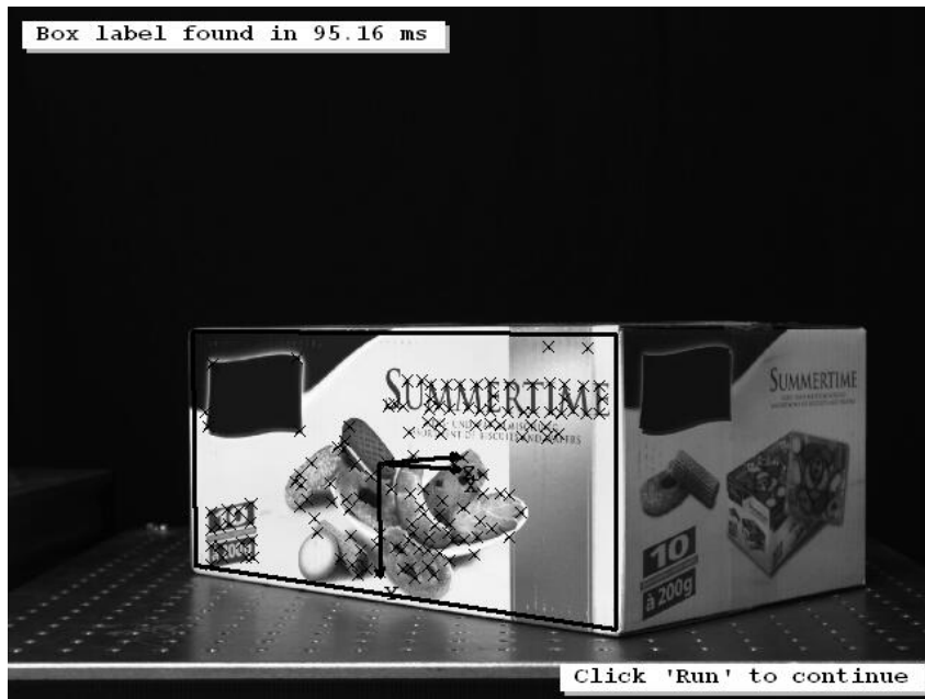
Figure 3.31: 3D pose of cookie box label obtained by calibrated descriptor-based matching.
