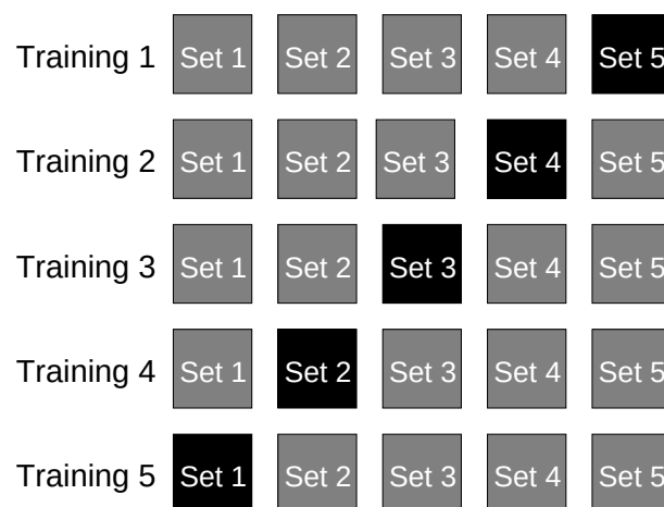
Figure 8.1: Cross validation: The training data is divided into 5 sub sets. Each set is used once as test data (black) that is classified by a classifier trained by the training data of the other 4 sub sets (gray).
